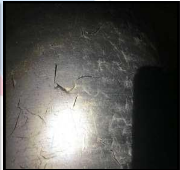
Figure 3. Gouge and Cuts on the Belt
